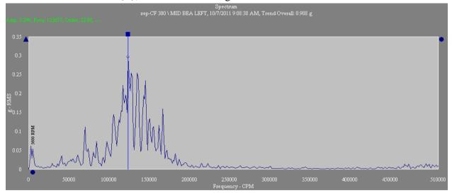
Vibration results: - Point (A), Side of mid bearing of vertical shaft
