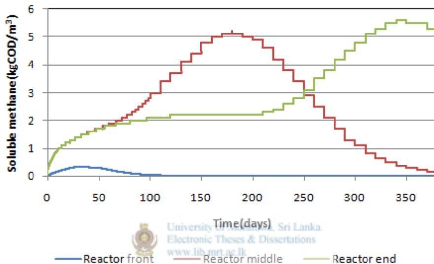
Figure 4-34: Concentration of soluble methane variation along the reactor under 360 days HRT
