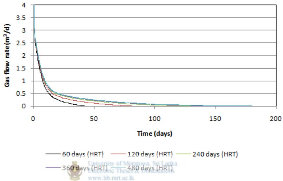
Figure 4-38: Gas production rate under different retention times
