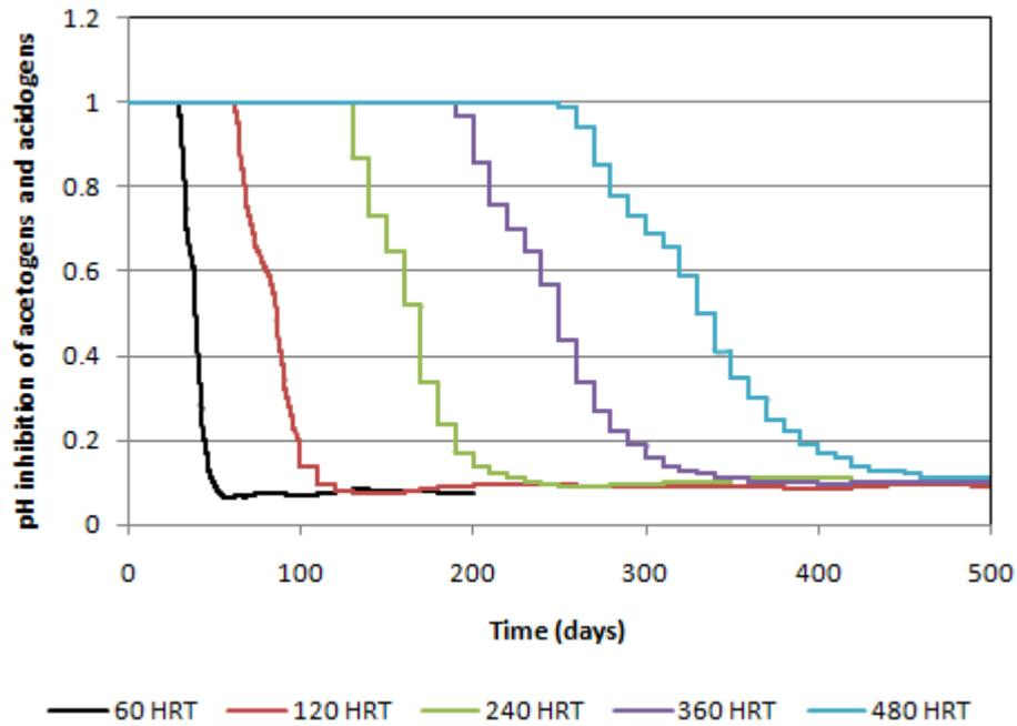
Figure 4-20: pH inhibition of acetogens and acidogens at reactor middle
