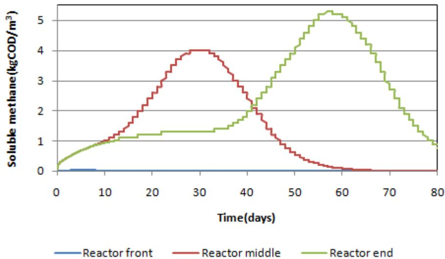
Figure 4-25: Concentration of soluble methane variation along the reactor under 60 days HRT
