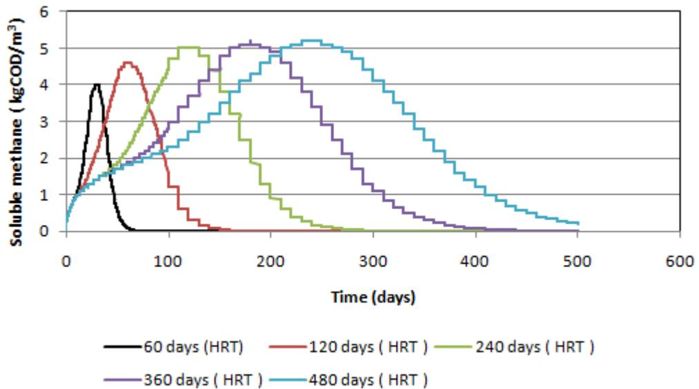
Figure 4-9: Dissolve methane concentration at the plug flow reactor middle
