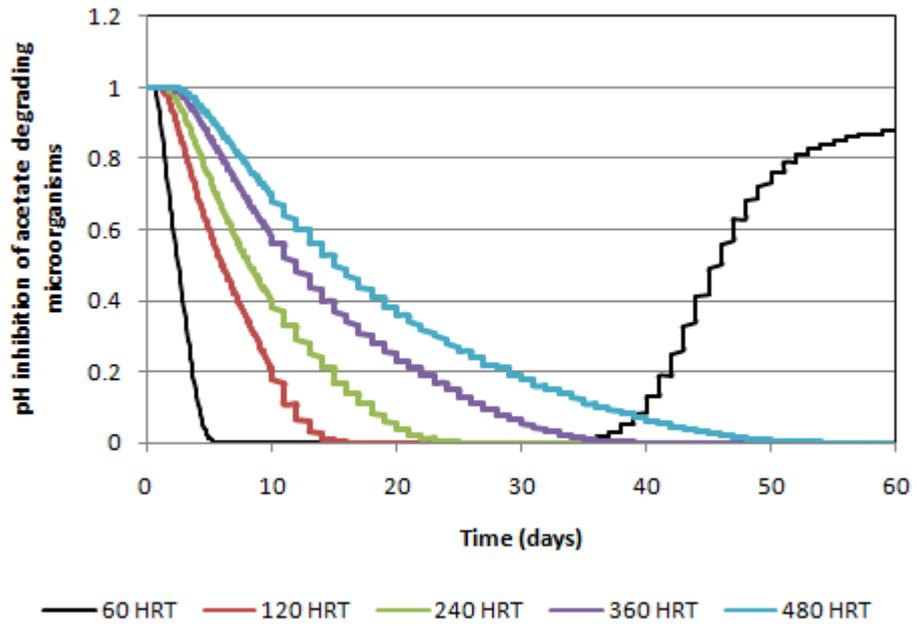
Figure 4-17 : pH inhibition of acetate degrading microorganisms at reactor front
