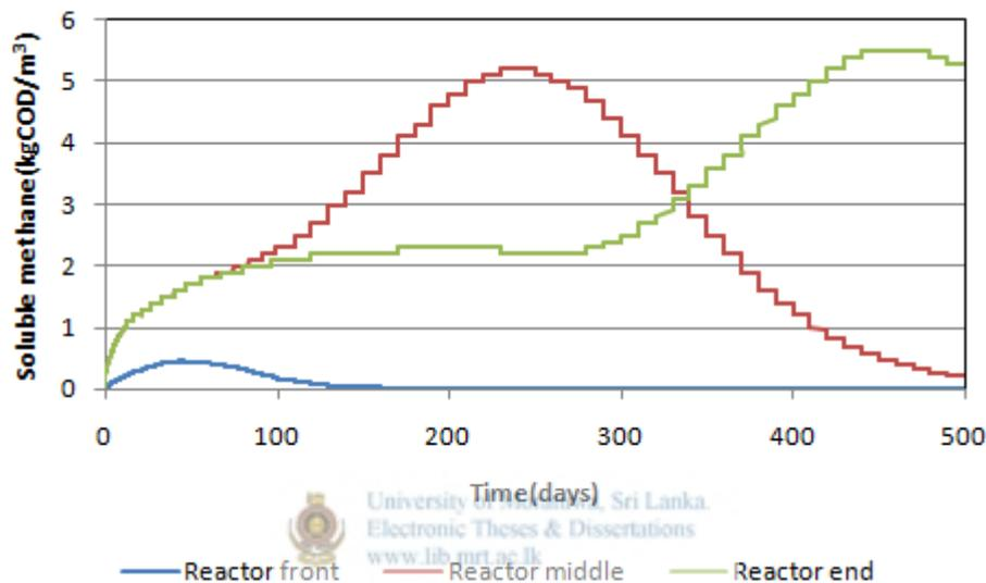
Figure 4-37: Concentration of soluble methane variation along the reactor under 480 days HRT
