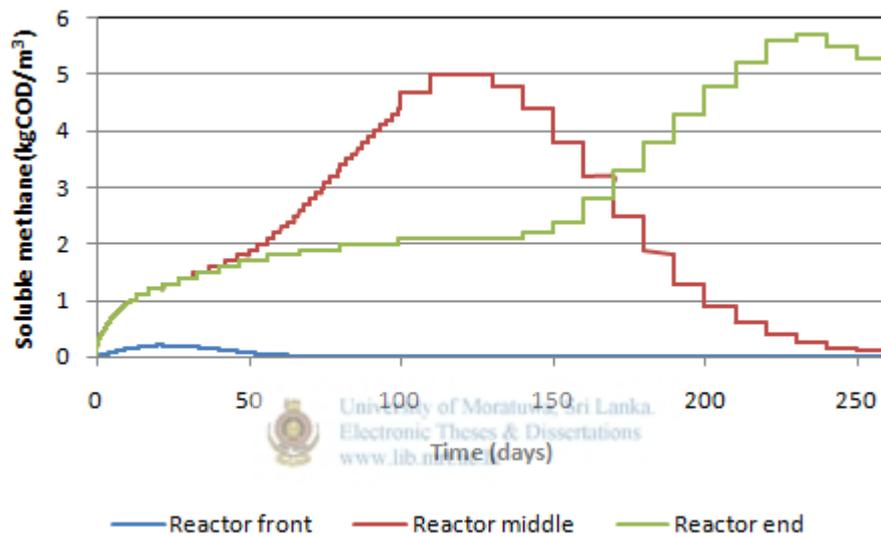
Figure 4-31: Concentration of soluble methane variation along the reactor under 240 days HRT
