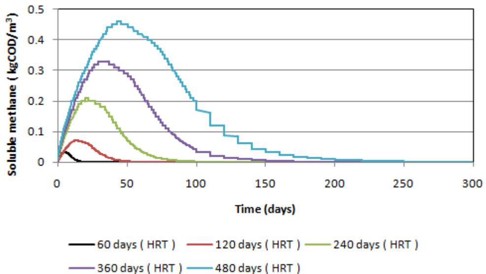
Figure 4-8: Dissolve methane concentration at the Plug flow reactor front
