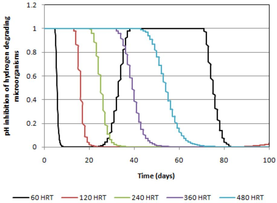
Figure 4-21: pH inhibition of hydrogen degrading microorganisms at reactor front
