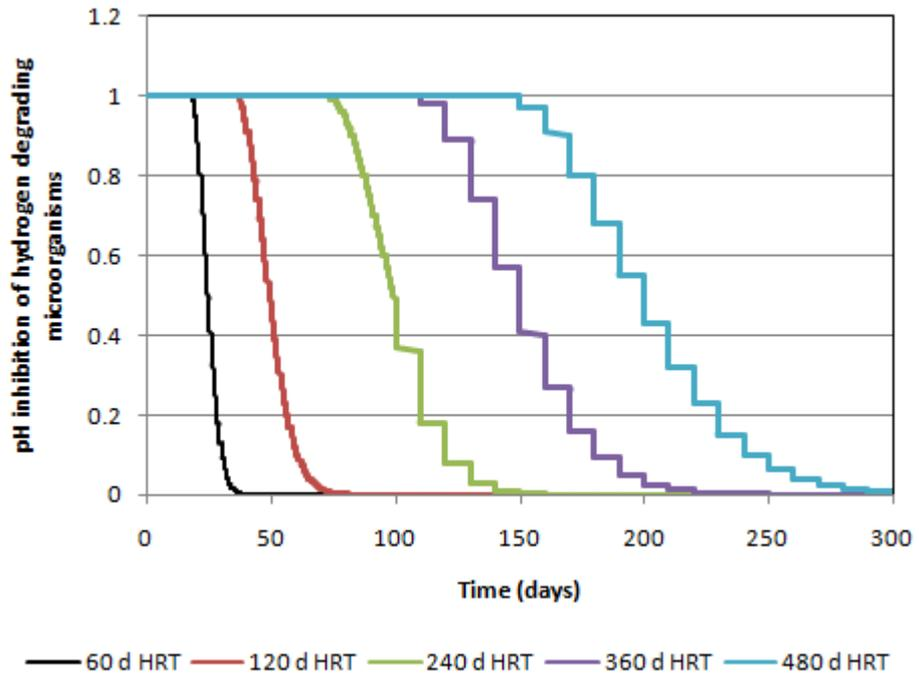
Figure 4-51: pH inhibition of hydrogen degrading microorganisms
