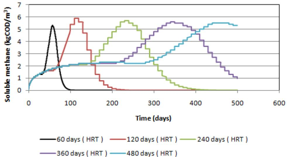
Figure 4-10: Dissolve methane concentration at the plug flow reactor end
