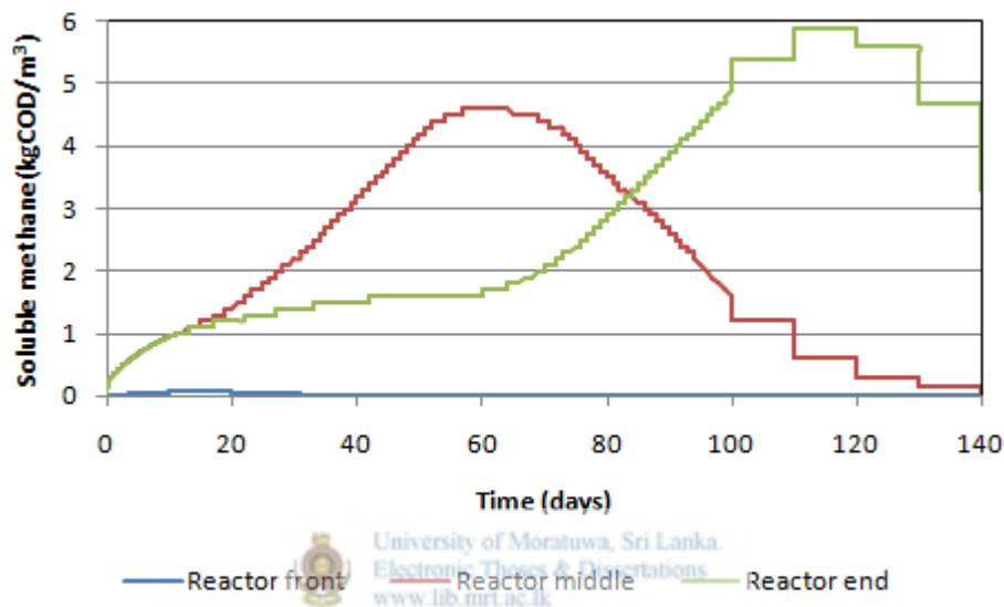
Figure 4-28: Concentration of soluble methane variation along the reactor under 120 days HRT
