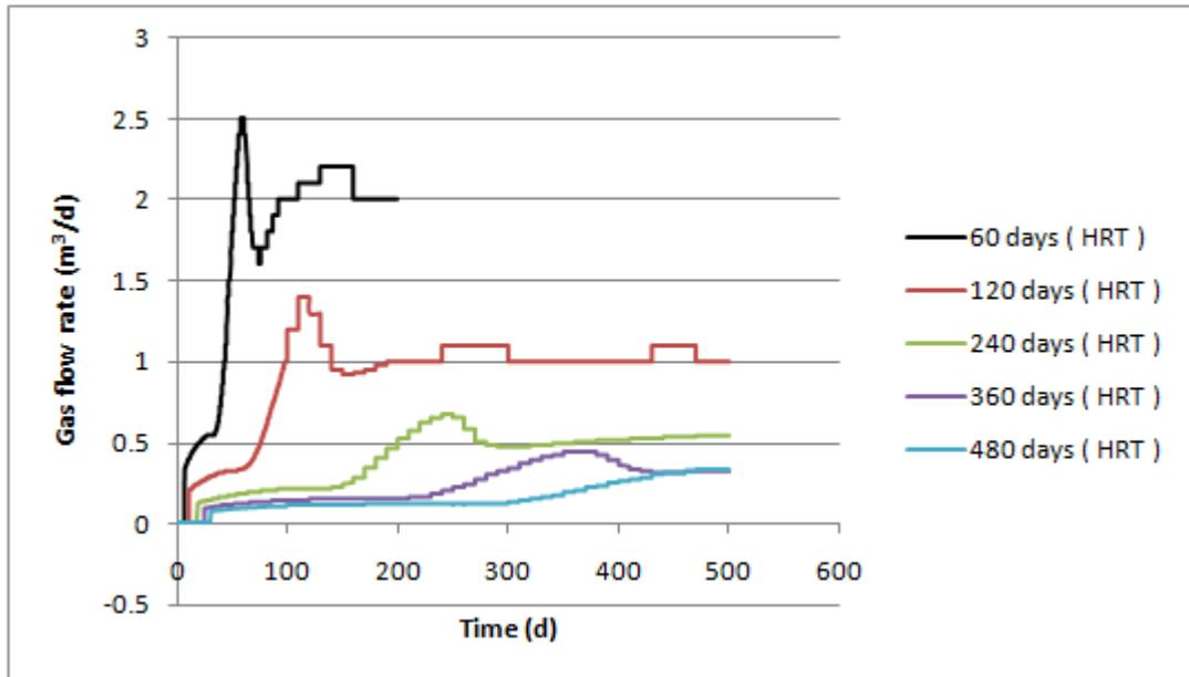
Figure 4-2: Variation of gas rate in PFR under different feed rates
