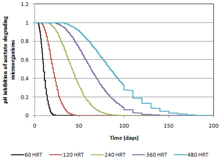
Figure 4-50: pH inhibition of acetate degrading microorganisms
