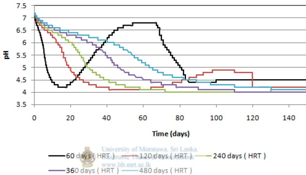
Figure 4-14: pH variation of the plug flow reactor at front
