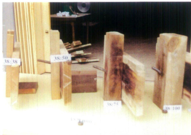
Figure 7.4: Different failure patterns observed for joints made with 15.9mm bolts – Perpendicular to grain loading – Ginisapu species ( Thickness details as shown in figure )
