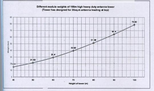
Figure 9.3a - Tower weight vs Height
