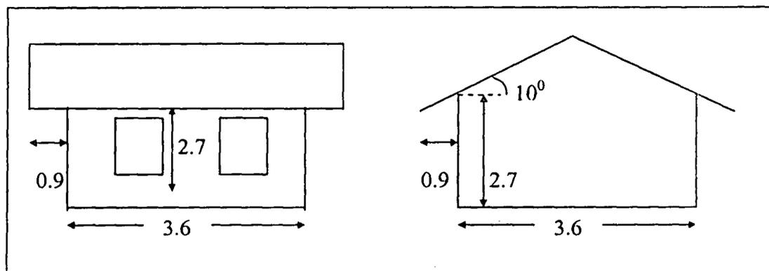
Figure 4.3: Front and side elevation of model house with east-west ridge roof
