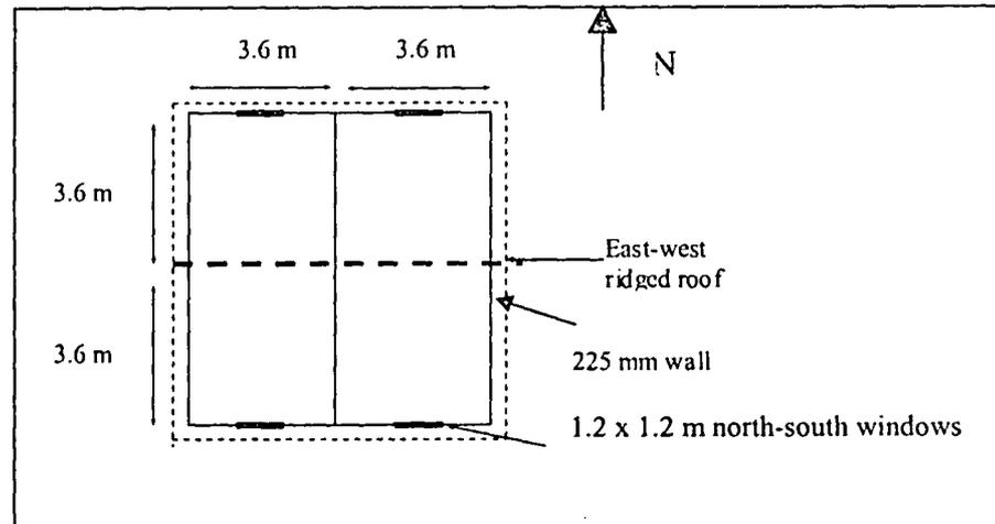
Figure 4.2: Floor plan of general case of the model house
