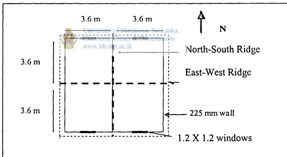
Figure 4.5: Roof Orientations
