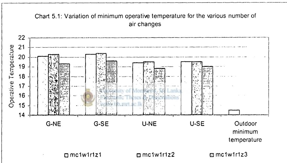
The infiltration of outside air could give rise to a certain number of air changes. The maximum and minimum operative temperatures for the three combinations of air changes are presented in Charts 5.1 and 5.2.
