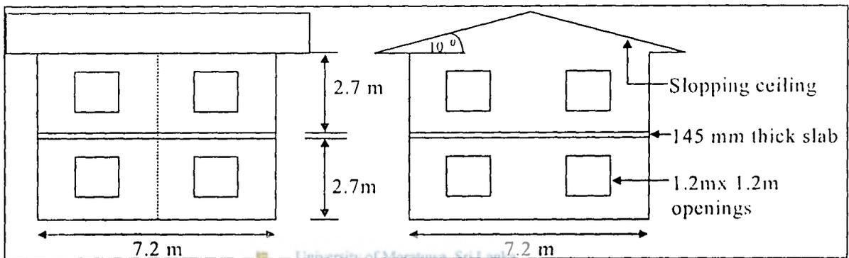
Figure 5.2: Front and side elevations of the model house
