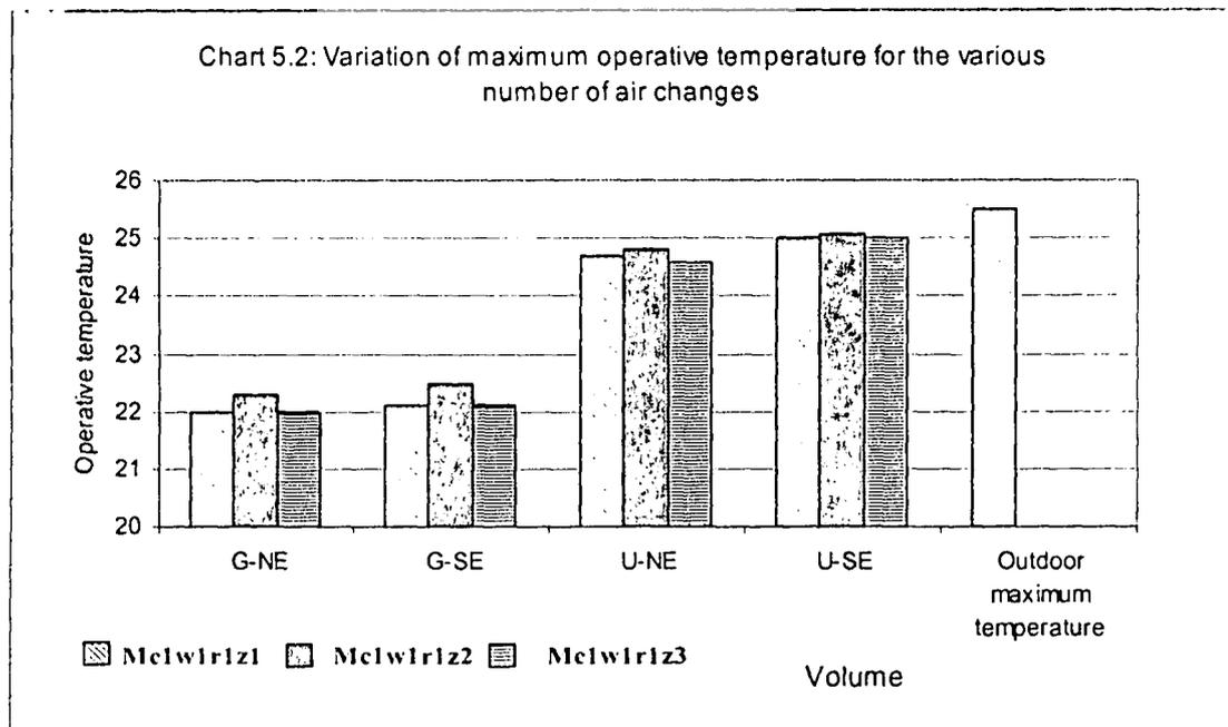
Chart 5.2 indicates that the infiltration has only a marginal effect on the indoor maximum operative temperature. The maximum temperature recorded by the ground floor is less than the upper floor. This may indicate that the upper floor areas could be better during the daytime as far as cold discomfort is concerned, except in days where hot discomfort will
