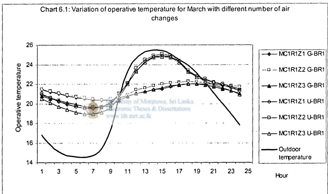
When the effect of infiltration is considered, the case which allow greater ventilation only during the daytime (Z2) gave a higher day time temperature for the ground floor. This is true for the upper floor as well. Thus, either Z1 or Z2 could be adopted in a well planned passive house. Z2 is more practical, since it allows the opening of some windows during daytime.
