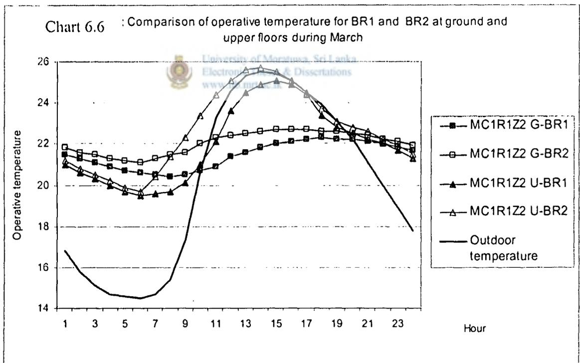
Chart 6.6 gives a comparison between bed room 1 and 2 at ground floor and upper floors. This could be used to determine the effects of various roof orientations in tropical uplands. It can be seen from Chart 6.6 that between 6.00 to 13.00 hours, there is a considerable difference in the bed room No 1 (BR1) and bed room No 2 (BR2) temperatures. This could be attributed to the window facing east. It would allow a considerable amount of direct solar radiation, during the morning.
