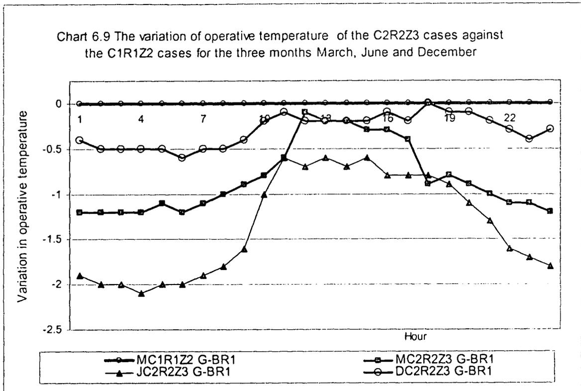
This also further reiterates the importance of curbing higher infiltration during the night with suitable construction techniques. In this context, provision of a ceiling is quite important for the upper floor and also some steps to reduce the ventilation of the roof void would be quite important.
