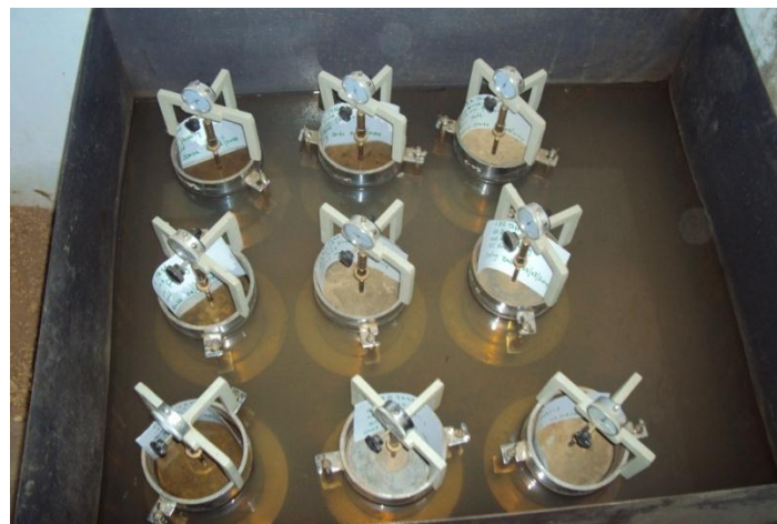
Figure 3.6: Immersed Soil Specimens in a water tank
