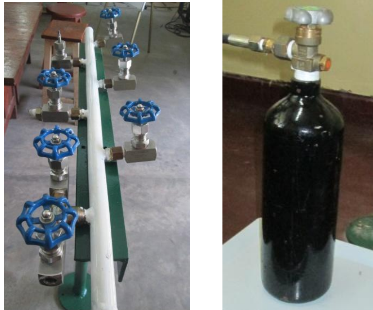
Figure 4.1 :Gas Manifold (Left) & Adsorption cylinder (Right)
