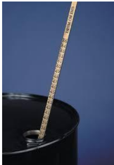
Figure 2.1: Level Measurement using Dipstick
