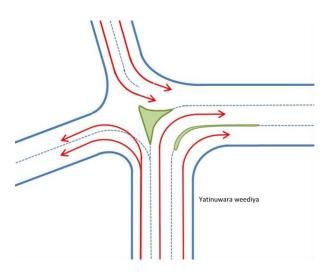
Figure 14: Introducing channelization near the junction
