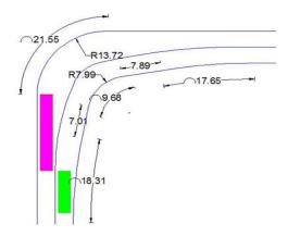
Figure 10: Proposed road curvature at meeramakkam junction
