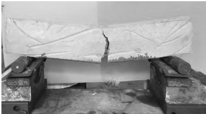
Figure B.2: Failure of specimen C(2)
