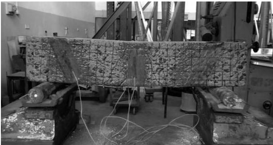
Figure B.7: Failure of specimen FA2(1)
