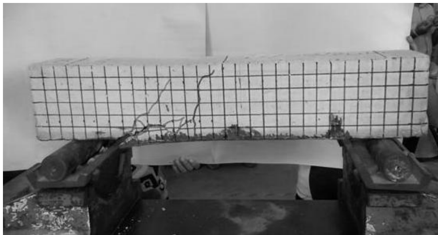
Figure B.4: Failure of specimen F(2)
