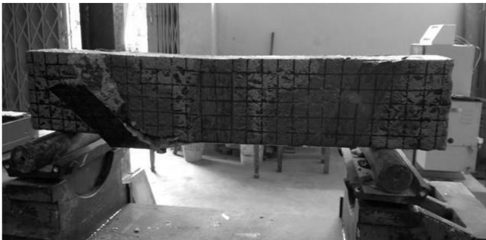
Figure B. 8: Failure of specimen FA2(2)
