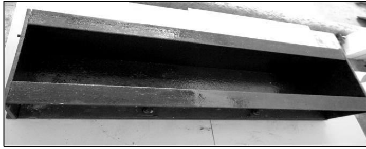
Figure 3.10: Steel mould for beams
