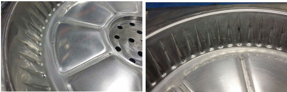
Fig 3.8 Worn out cavities (Source: Dana Tool Room WLL)
