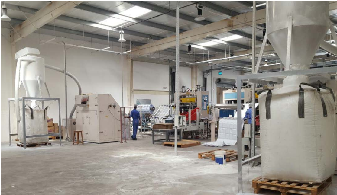
Fig 3.24 After Crushing Recycles collected to Bags via Cyclone Separator (Source: Dawanco Ind WLL)
