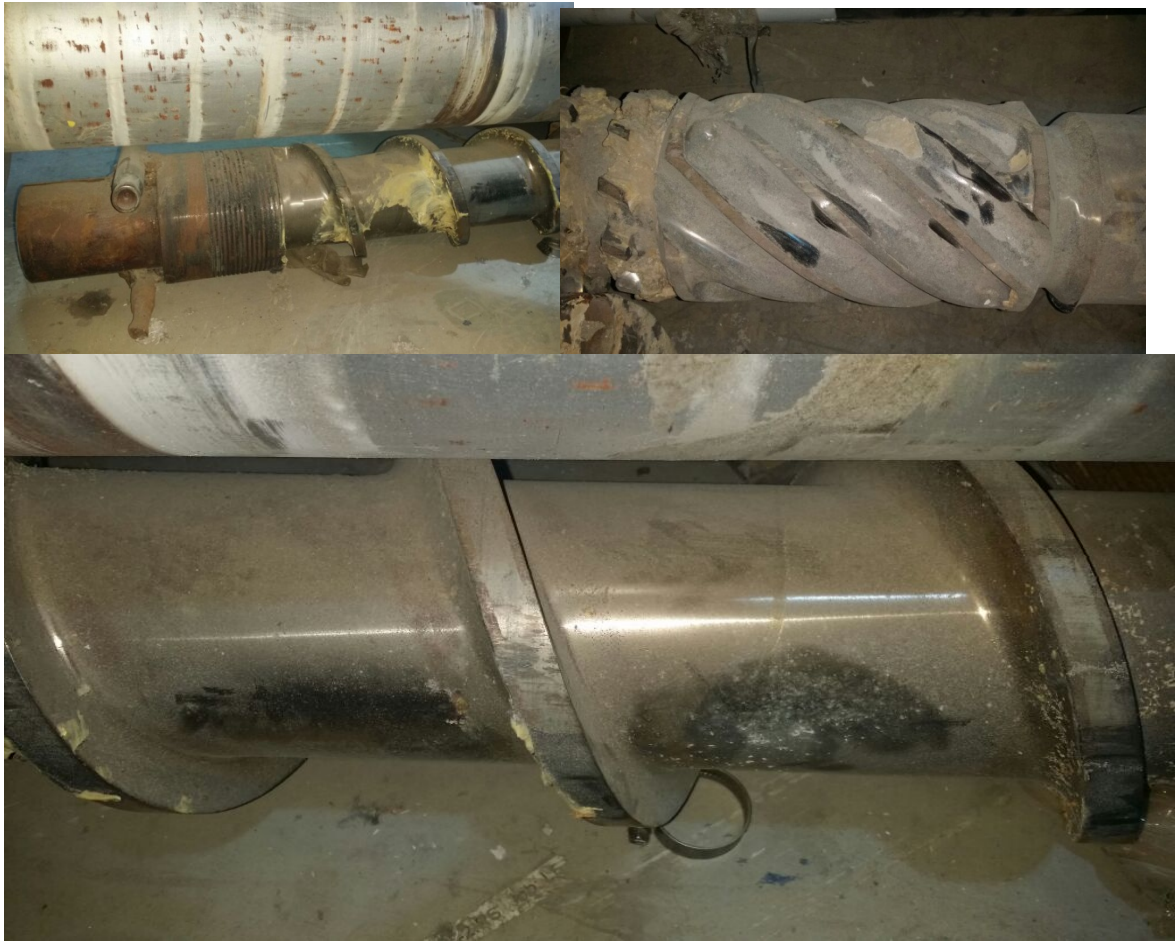
Fig 3.9 Worn out screws(Source: Dawanco Ind. WLL)
