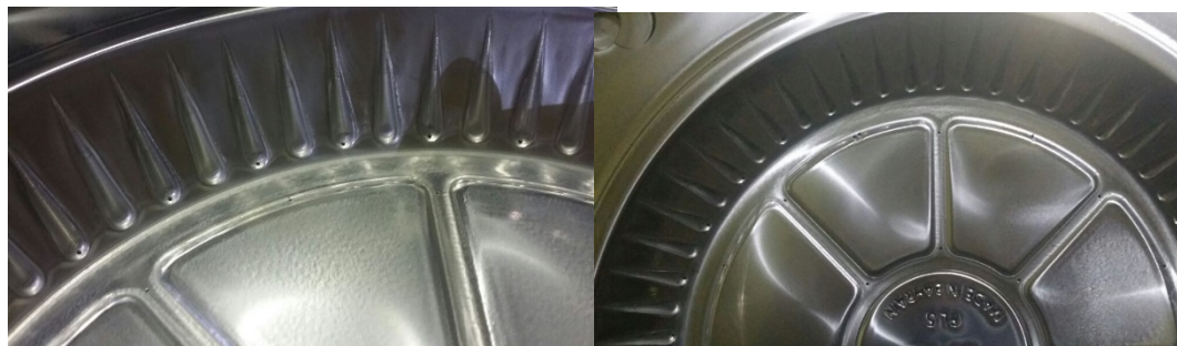
Fig 3.15 Vacuum Forming Mold Cavities with Vent holes (Source: Dana Tool Room Wll)
