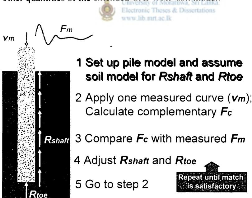
Figure 3.2 CAPWAP Data Analyses Procedure
