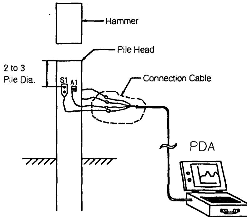
Figure 3.1 Instrumented pile
