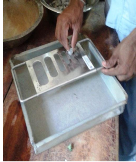
Figure 6: Performing FI test
