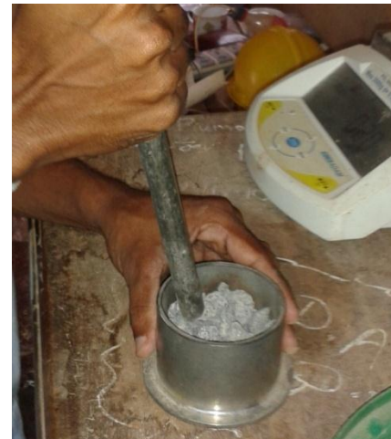
Figure 5: Aggregate for AIV test
