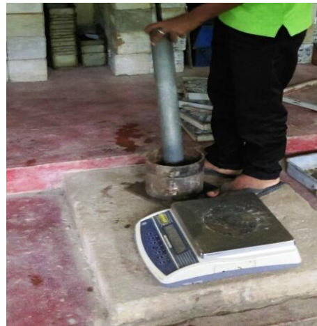
Figure 11: Casting ABC specimen
