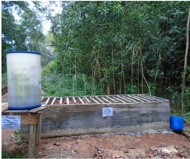
Figure 3.3: Front view of the HSSF sectioned into columns and planted with Phragmites karka
