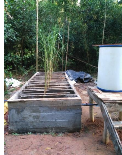
Figure 3.4: Side view of the HSSF planted with Phragmites karka in the mid of the each section
