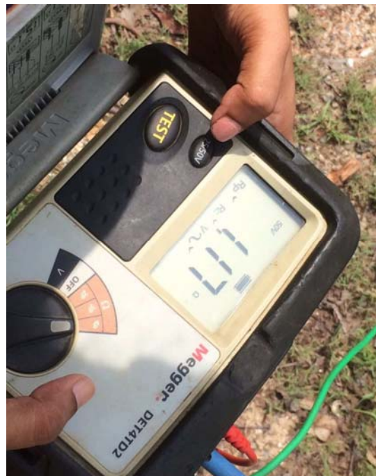
Figure 5.15 -Resistivity Reading at the Site
