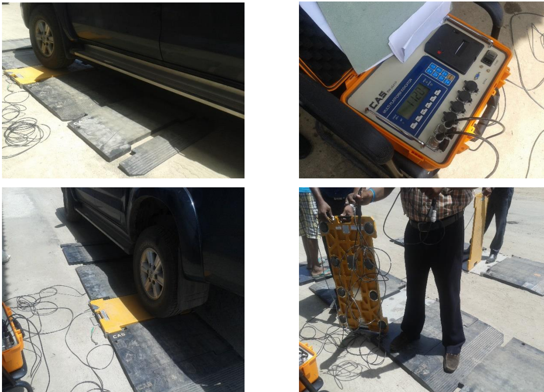
Figure 3-1; Measuring of axle weight of a vehicle
