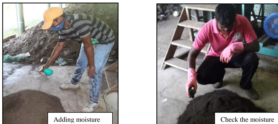
Figure 21 - Moisture content adjustment by addition of water
