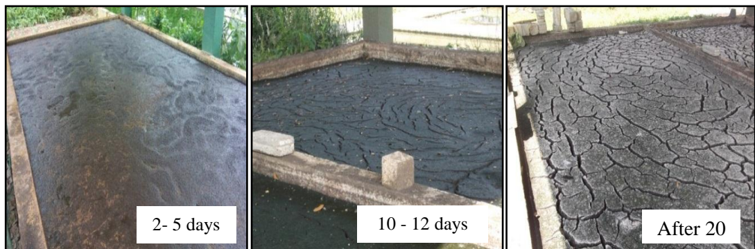
Figure 15 - Drying stages of FS in the sand bed
