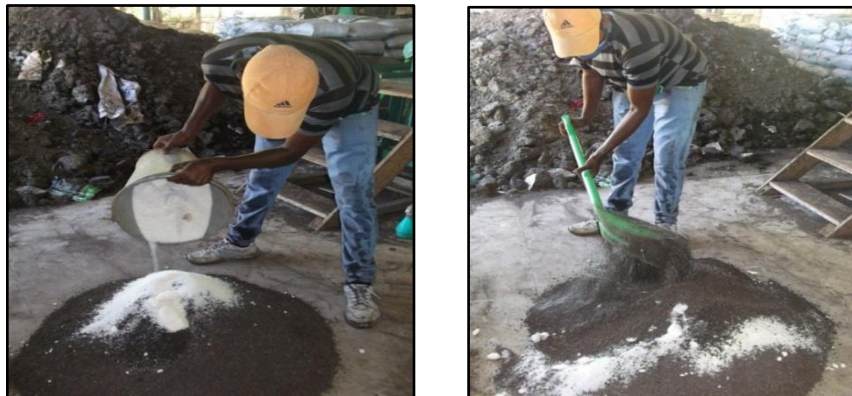
Figure 22 - Adding binding agents and mixing
