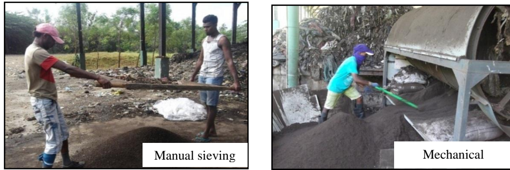
Figure 20 - Compost sieving of manual and mechanical method
