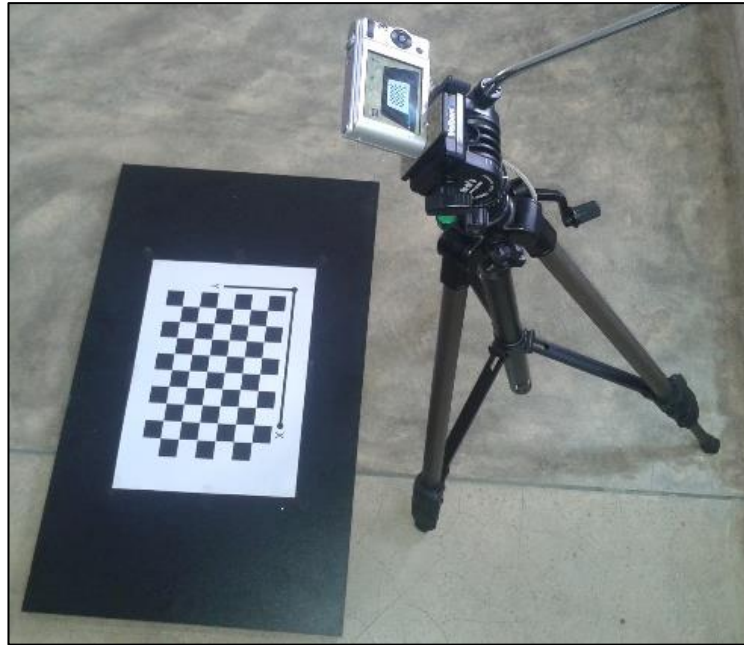
Figure 3.7: Experimental setup of camera calibration
