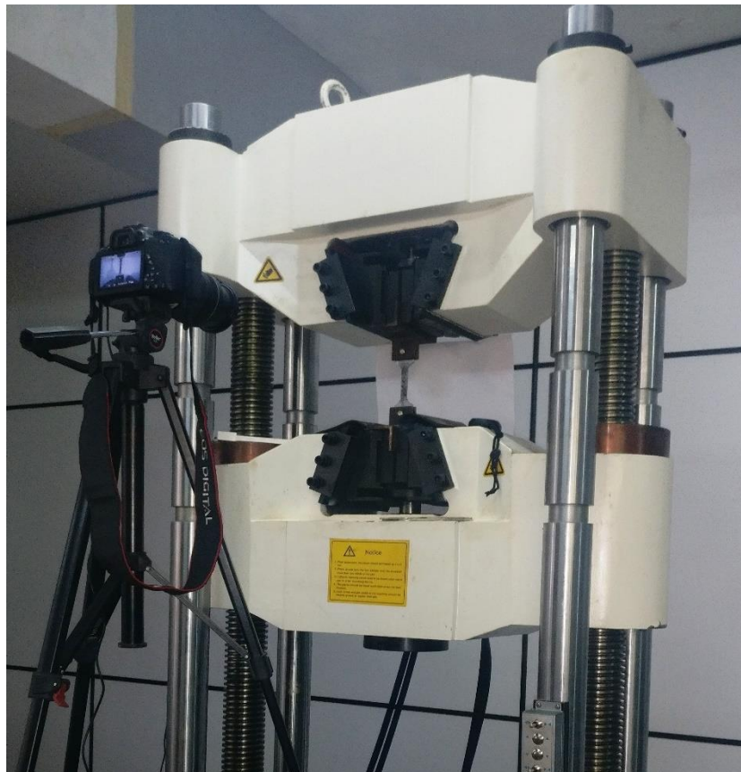
Figure 5.7: Experimental setup of uniaxial tensile testing
