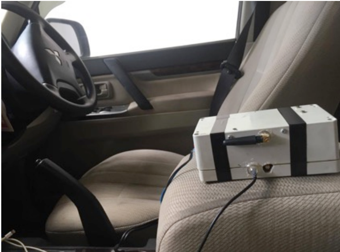
Figure 24: GPS Device mounted in a probe vehicle
