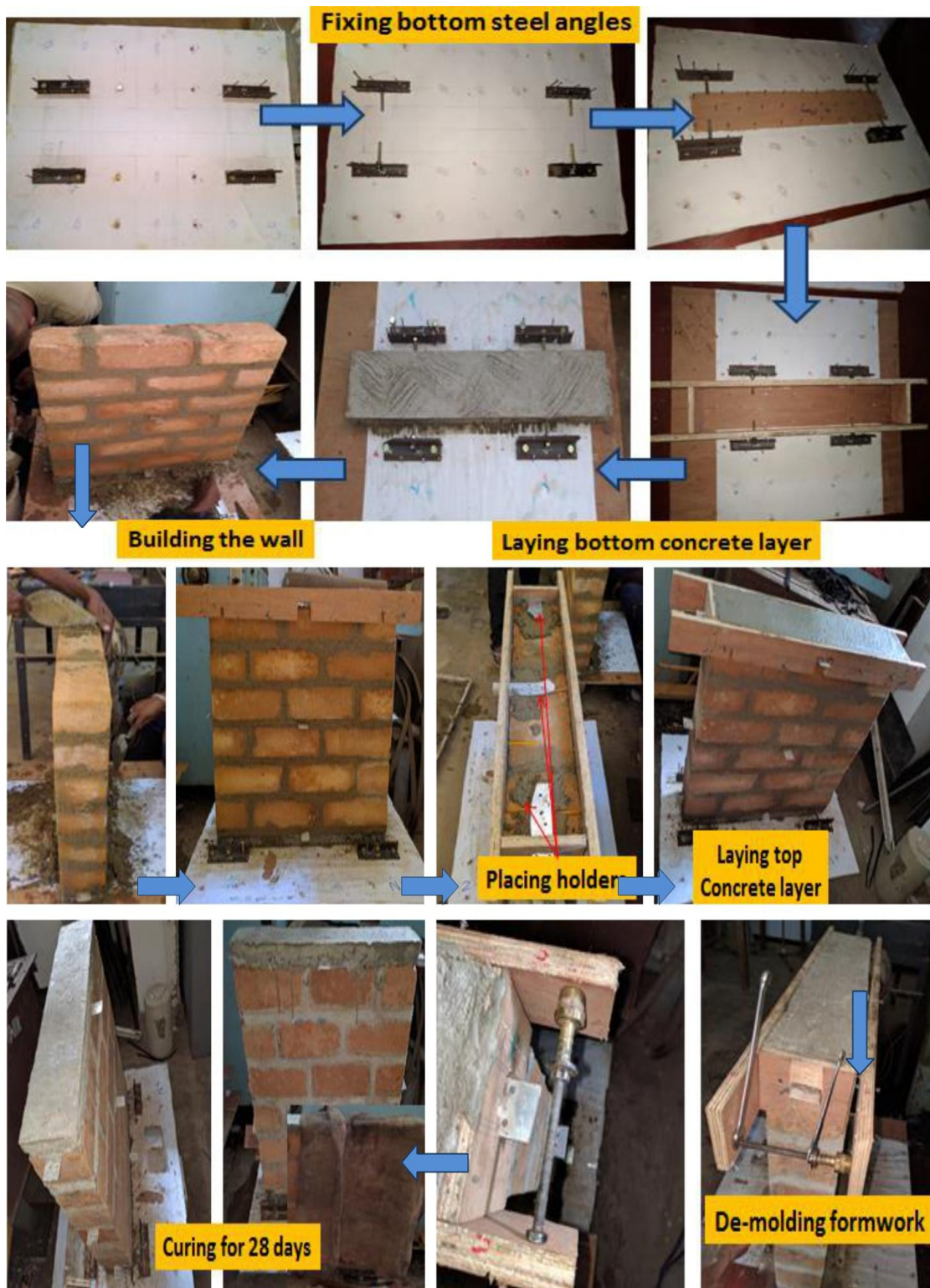
Figure 3.7: Construction steps of CSEB wall panel
