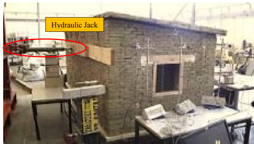
Figure 2.10: Load application using hydraulic jack
