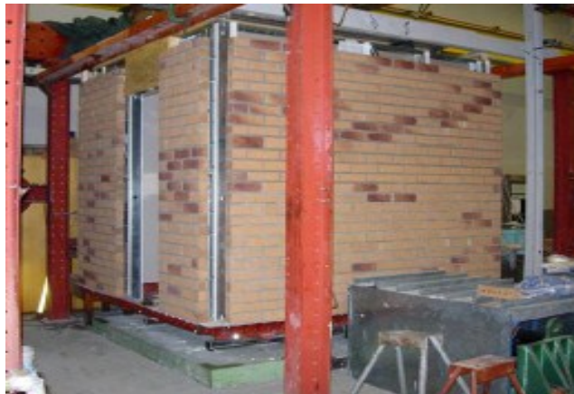
Figure 2.2: Experimental set up with steel frames
