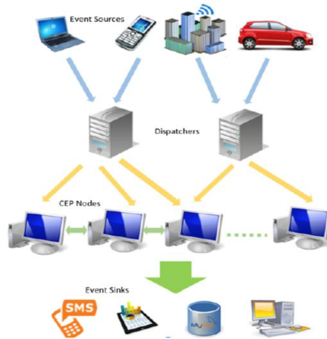
Figure 2-5 VISIRI high-level system architecture [8]
