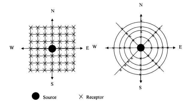
Figure 3.4: Cartesian receptor grid Figure 3.5: Polar receptor grid
