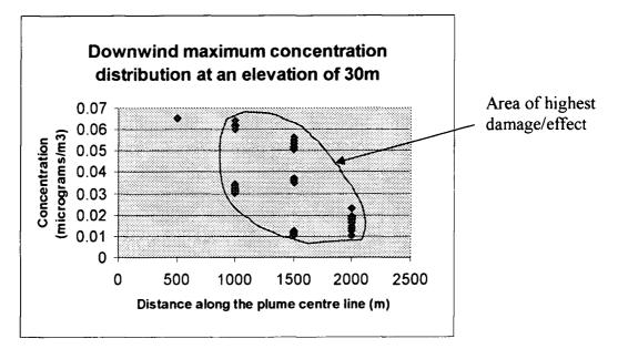
Figure 4.2: Maximum Concentration at a 30m Elevation for an Emission from a Stack Height 80m and Plume Exit Velocity 20m/s
