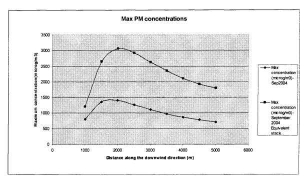
Figure 4.11: Distribution of maximum ground level concentrations of particulate matter
