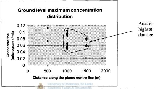
Figure 4.5: Maximum concentration points at ground level for an emission from a stack height 50m and wind velocity 20m/s
