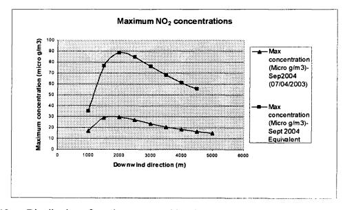
Figure 4.12: Distribution of maximum ground level concentrations of NO<sub>2</sub>
