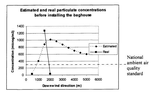
Figure 5.1: Estimated and real particulate concentrations before installing the baghouse
