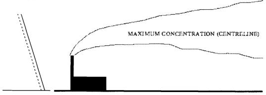
Figure 2.9: Coning Plume
