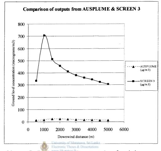
Figure 5.3: Predicted ground level; concentration of particulate matter using AUSPLUME and SCREEN 3
