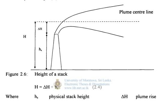
The plume rise is the increase in the height due to the momentum and the buoyancy effects of the plume. The momentum component is the rise due to the physical speed at which the effluent is released and the buoyancy is due to the thermal characteristic of the plume relative to the ambient air.
