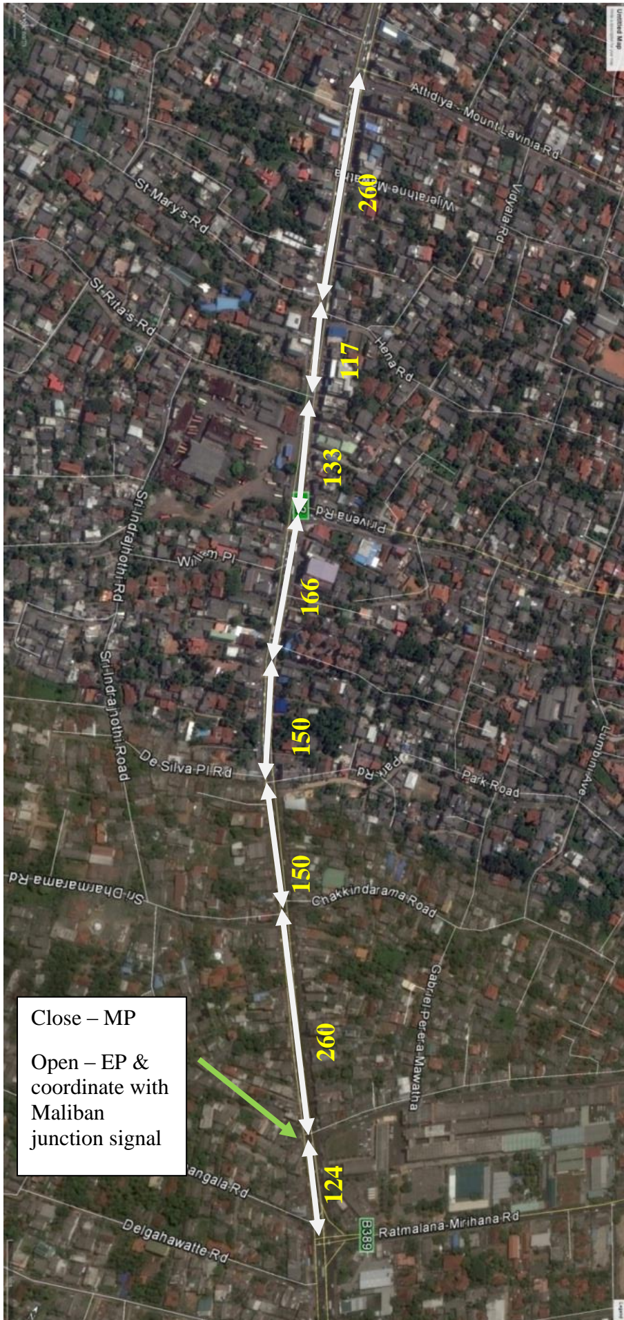
Figure 5-7 Finalized Opening Locations and Spacings
