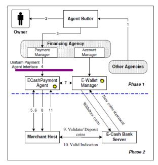
Figure 2.3: Entity Interaction diagram for an E-Cash Payment Transaction
