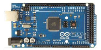
Figure 2-20 Arduino Mega 2650
