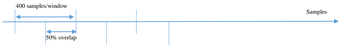
Figure 64: Moving window with 50% overlap
