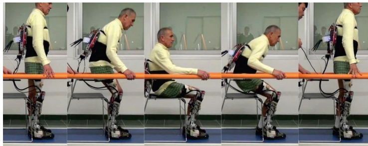
Figure 2.10: CYBERLEGS Beta-Prosthesis: An active lower limb ortho-prosthesis at work [15]
