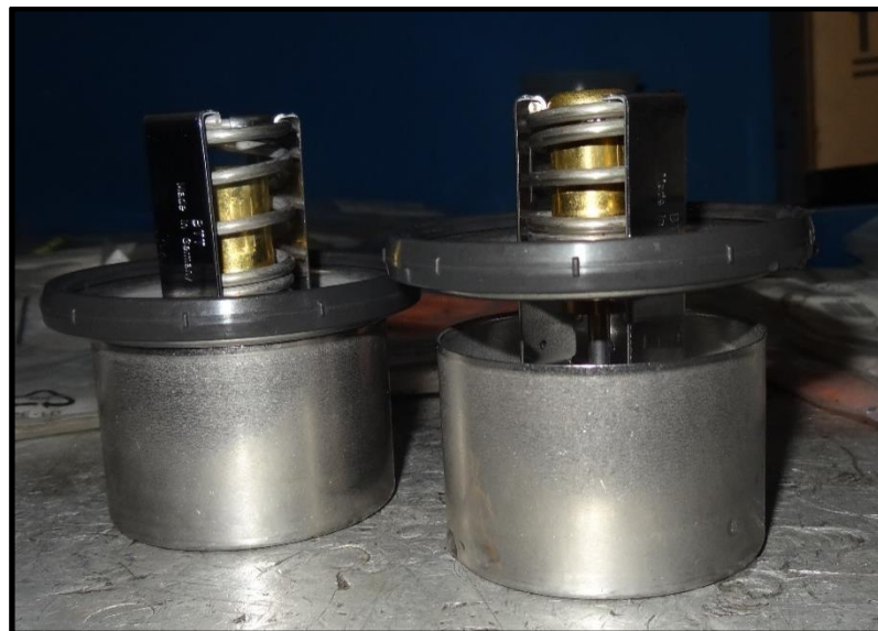
Figure 2.19: Thermostat of DEUTZ TBD 620
