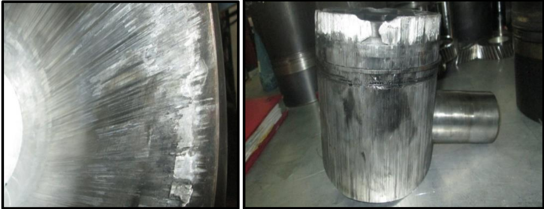
Figure 2.1: Cylinder Liner and Piston subjected to heavy seizure
