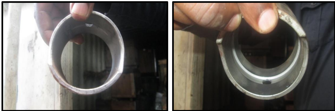
Figure 2.6: Initial Bearing and Upgraded bearing
