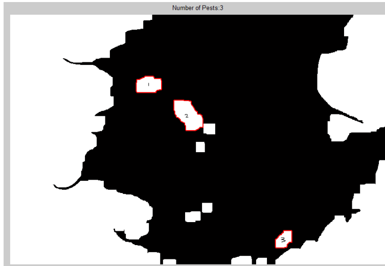
Figure 11: Pest regions detected from the binary image
