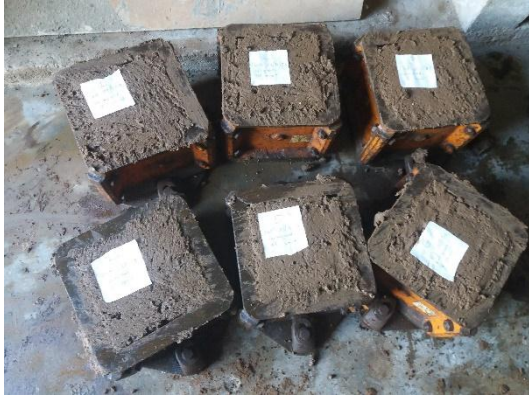
Figure 13-Soil cubes are ready for compressive strength testing in dry condition
