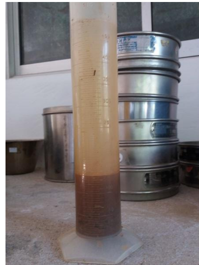
Figure 4- Soil kept undisturbed for sedimentation
