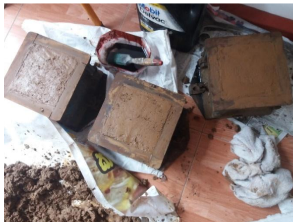
Figure 25- Cube casting for Mud concrete at site mix used at site
