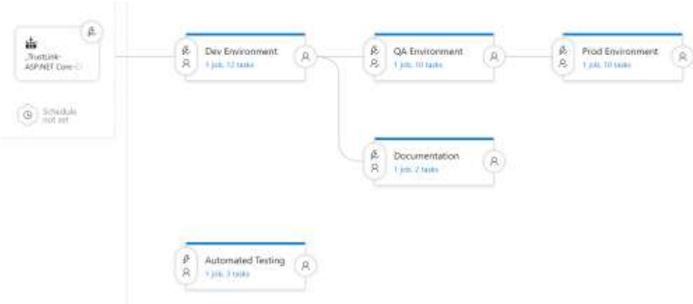
Figure 5.3.4: Release Pipeline after Adding SDM
