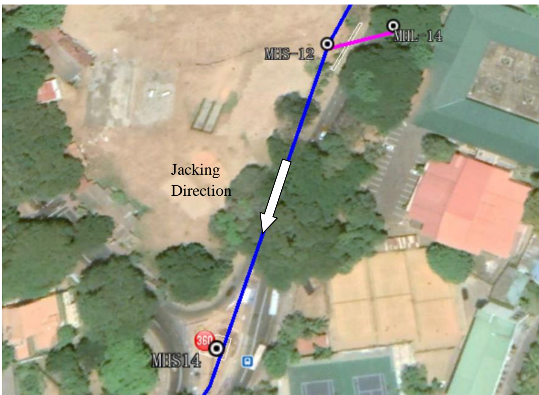
Figure 45 Jacking alignment of Torrington Tunnel
