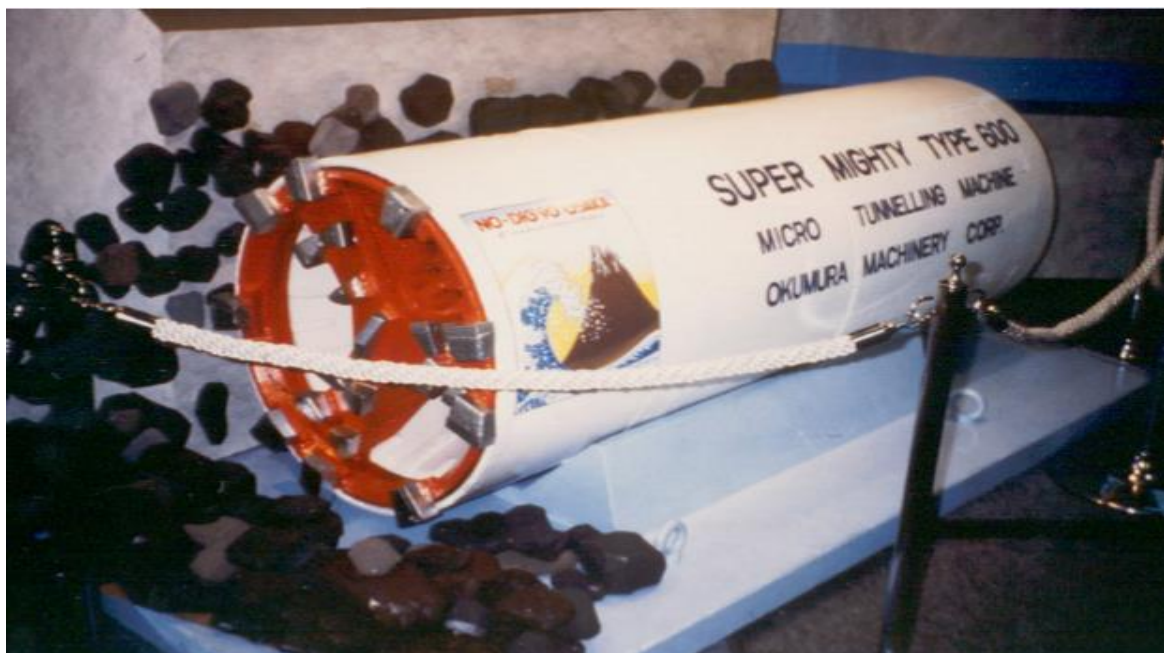
Figure 12 - Microtunnel boring machine (MTBM)
