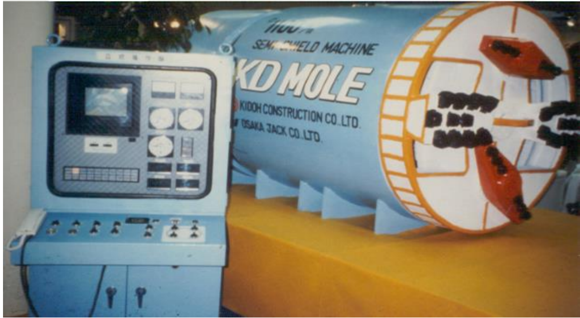
Figure 13 - Micro tunnel boring machine (MTBM)
