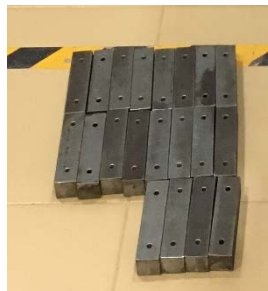
Figure 4-11- External mass attached to the framed structure for irregularity conditions
