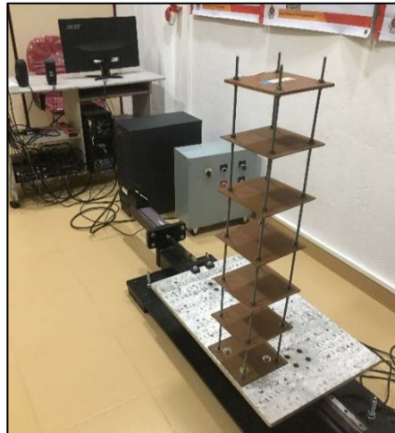
Figure 4-1 Shaking table (ANCO R-201) in Department of Civil Engineering, University of Moratuwa
