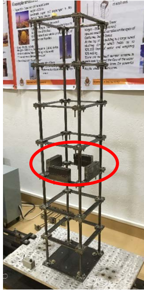
Figure 4-15 Mass irregularity imposed on the 3rd storey in the experimental model, mounted on the shaking table
