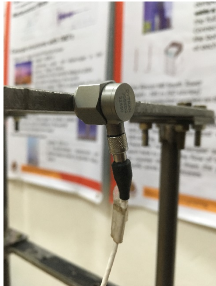
Figure 4-10- Accelerometer sensor connection to the slab using threaded holes to ensure zero relative movement
