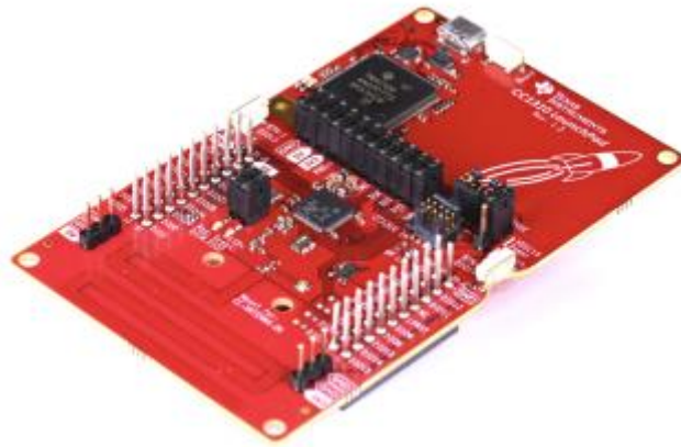
Figure 3.8. Texas instruments CC1310 Development board Source: Texas instruments official website
