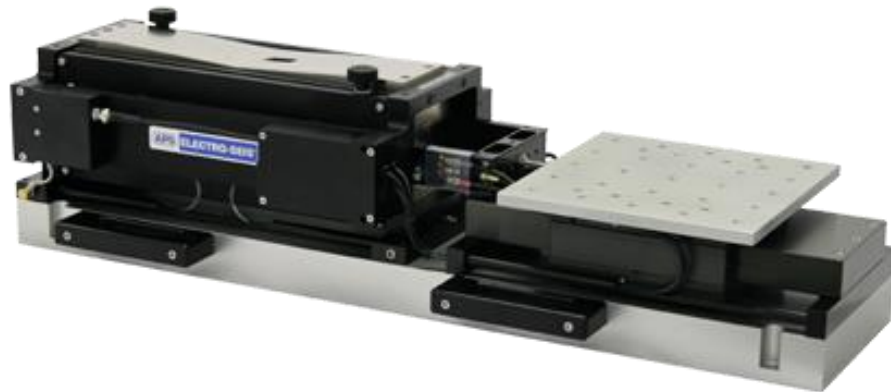
Figure 3.22. Shaker table Source: APS Dynamics official website
