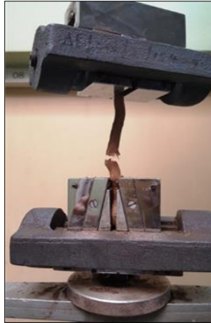
Figure 5.27 Root tensile strength testing using Dynamometer
