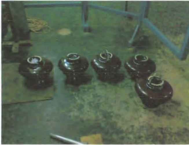
Figure 4.3 Sample Insulators before Testing
