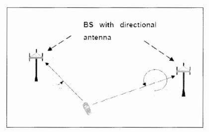
Figure 2.2: Angle of arrival parameter in GSM Source: [29]
