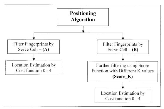
Figure 3.10: Different approaches of Positioning Algorithm
