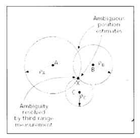
Figure 2.3: Propagation Time measurement Source: [18]
