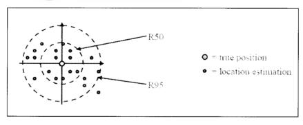
Figure 2.6: Circular Error Probability Source: [36]
