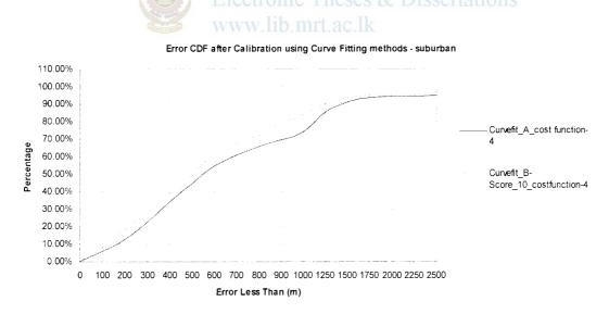
Figure 5.53: Positioning error CDF after calibration using curve fitting methods – Suburban
