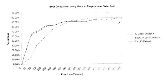
Figure 5.27: Error comparison using measured fingerprints - Galle Road
