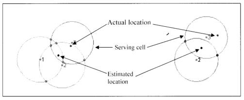
Figure 2.5: Geometrical mean of all intersection points in geometrical method Source: [29]
