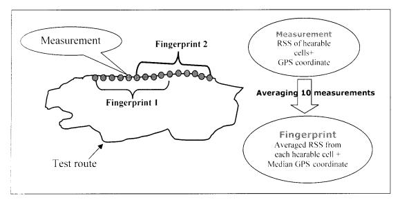
Figure 3.6: Methodology of fingerprint creation for measured database - Sliding Window
