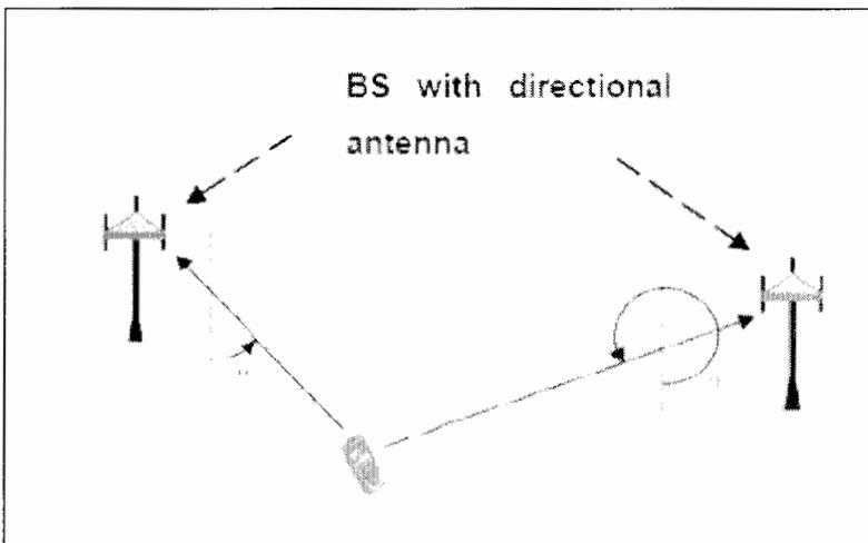
Figure 2.2: Angle of arrival parameter in GSM
