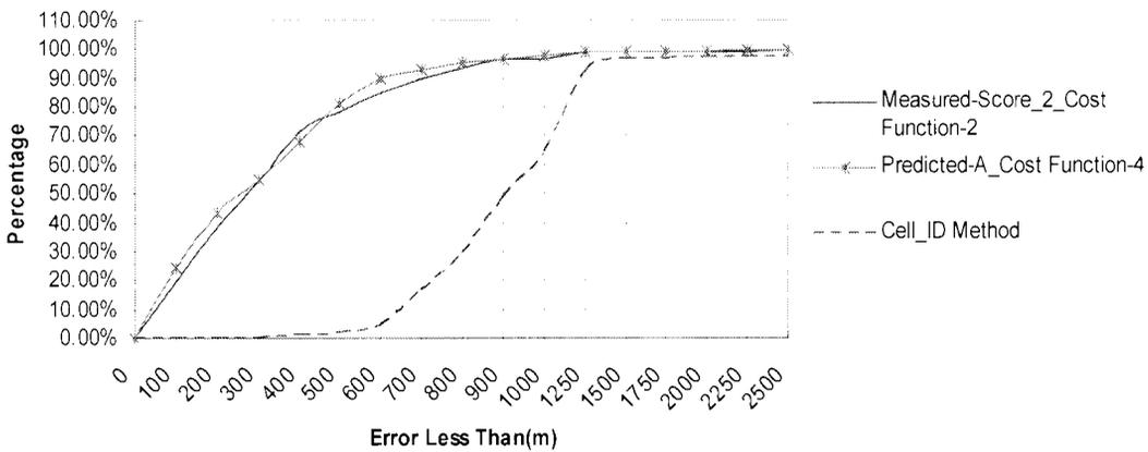
Figure 5.40: Error comparison using measured and predicted fingerprints - Rural
