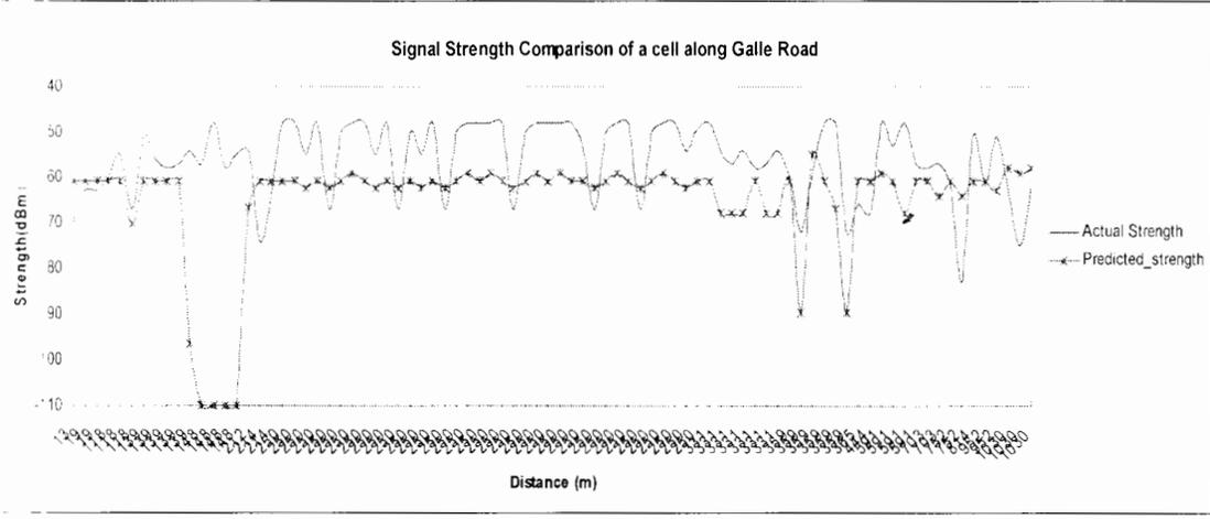
Figure 5.2: Signal Strength Comparison of a cell along Galle Road
