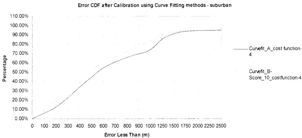
Figure 5.53: Positioning error CDF after calibration using curve fitting methods – Suburban
