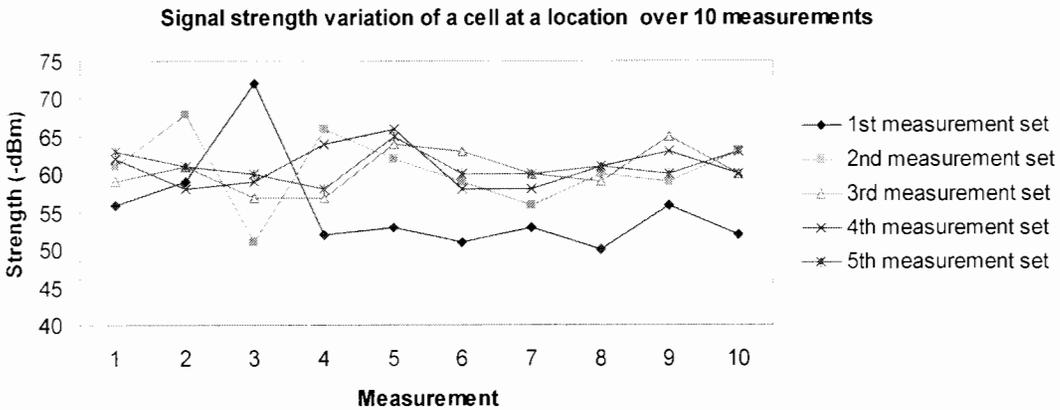
Figure 4.3: Signals strength variation of a cell at a location over ten measurements
