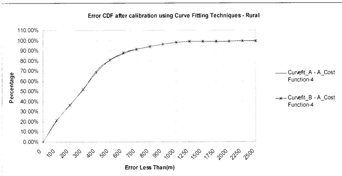
Figure 5.55: Positioning error CDF after calibration using curve fitting methods – Rural
