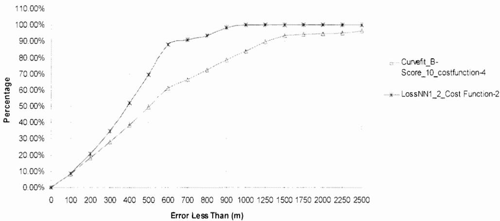
Figure 5.59: Performance comparison of curve fitting & neural networks for calibration – Suburban
