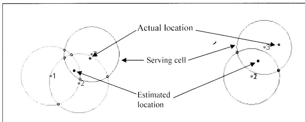
Figure 2.5: Geometrical mean of all intersection points in geometrical method
