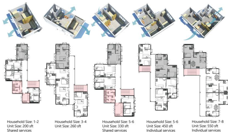
Figure 6, Illustrated proposed Plan for different dwelling type according to BNBC and income group
