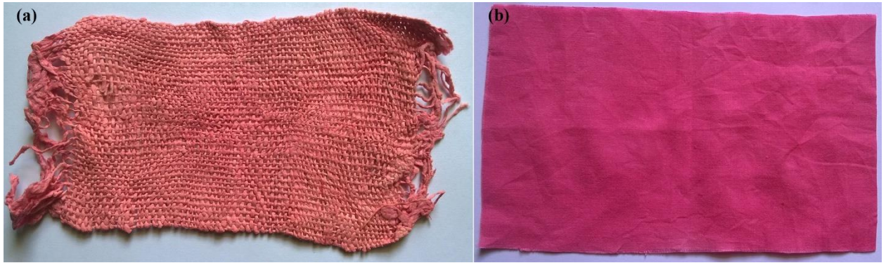
Figure 3.9: Dyed textile samples in dry condition (a) Dried after dyeing - LS samples, (b) Dried after dyeing - Cotton samples
