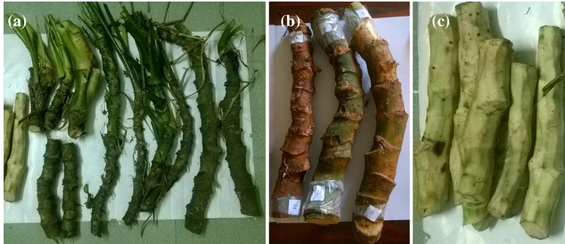
Figure 3.2: LS rhizome preparation for fibre extraction (a) pointy spines, (b) Separated rhizomes into different maturity levels, (c) Pointy spine and mud removed rhizomes
