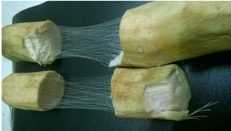
Figure 3.3: Mechanical fiber extraction from split rhizome
