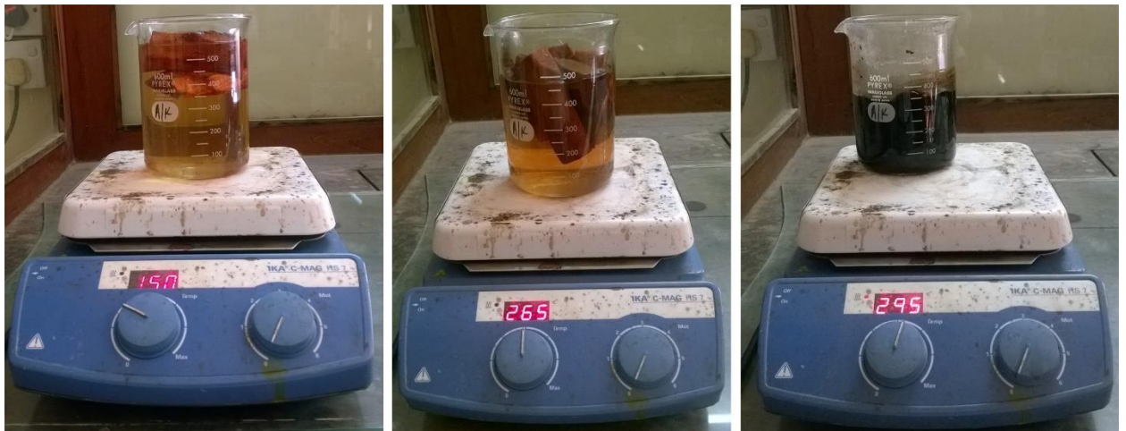
Figure 3.4: Alkali extraction of LS Rhizome fibre
