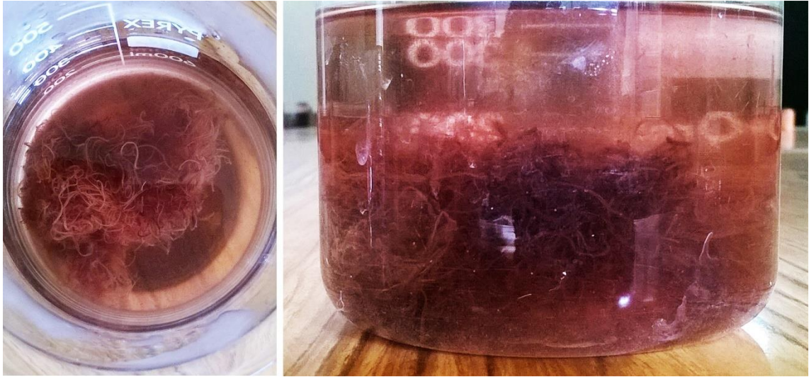
Figure 3.5: Alkali extracted rhizome fibre
