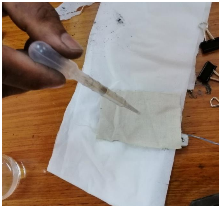
Figure 3.2.5 Inject electrolyte solution on the porous separator
