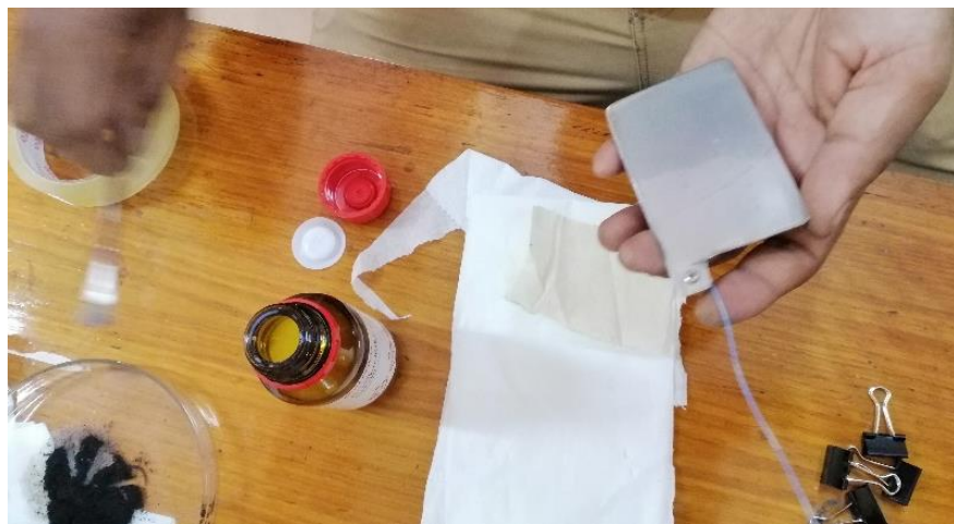
Figure 3.2.2 Applying adhesive solution on the stainless steel plate
