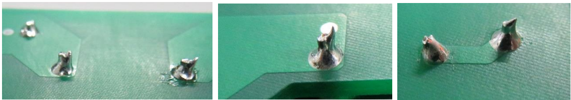
Figure 7.19: Deformations occurred on solder joints due to the wrong angle between soldering iron and vertical plane
