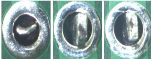
Figure 8.13: Different shapes of component leads
