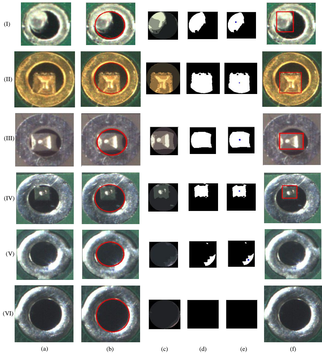
Figure 4.11: Detected component lead top inside the drill-hole region of the solder pad. (a). Extracted solder pad region. (b). Identified drill-hole region. (c). Resulted image after colour clustering. (d). Resulted image after thresholding and morphological filtering. (e). Computed centre point of the largest contour. (f). Solder pad image with detected component lead top. (I). Tin plated lead with ellipsoidal shape. (II). Gold plated lead. (III). Lead with highly illuminated areas. (IV). Lead with darker colour. (V). Empty solder pad with reflected light inside drill-hole. (VI). Empty solder pad with no reflected light
