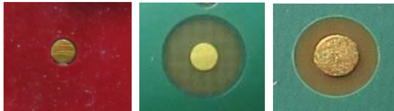
Figure 2.1: Fiducial points defined by the PCB layout designer
