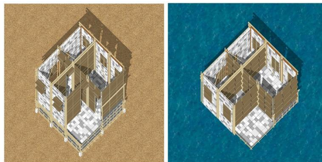
Figure 13, Wall Adaptability with water rise (normal-left, flood-right) (Source: Author)
