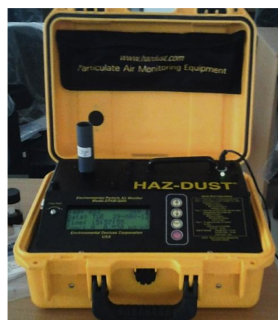
Figure 1.5: Haz-Dust Particulate Air Monitoring Equipment
