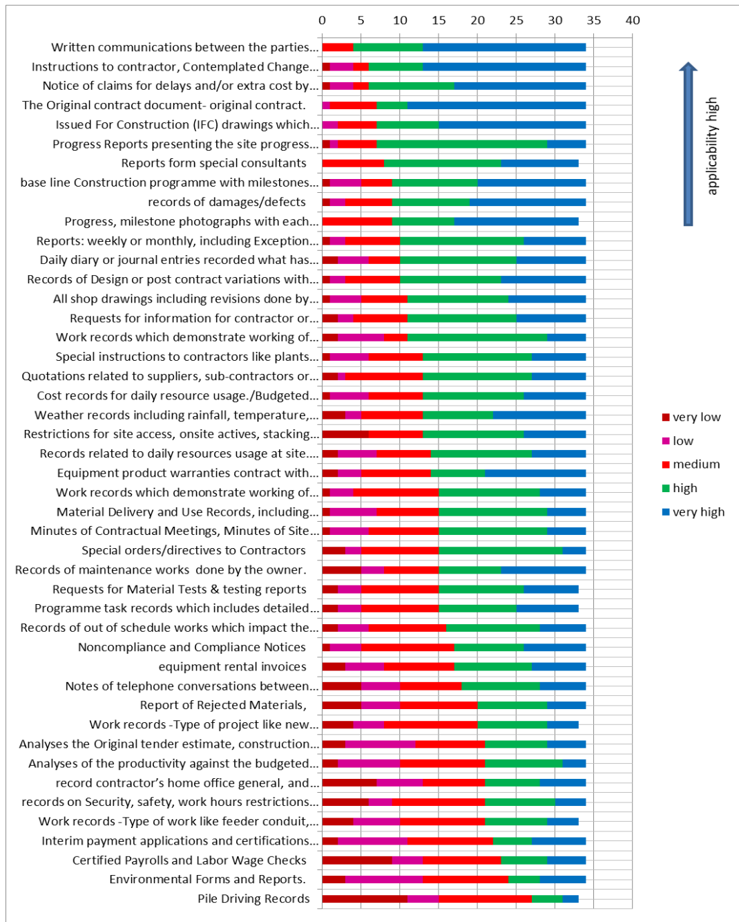
Figure 4.7: Applicability of different record types to manage the MEP claims in the Defect Liability Period.
