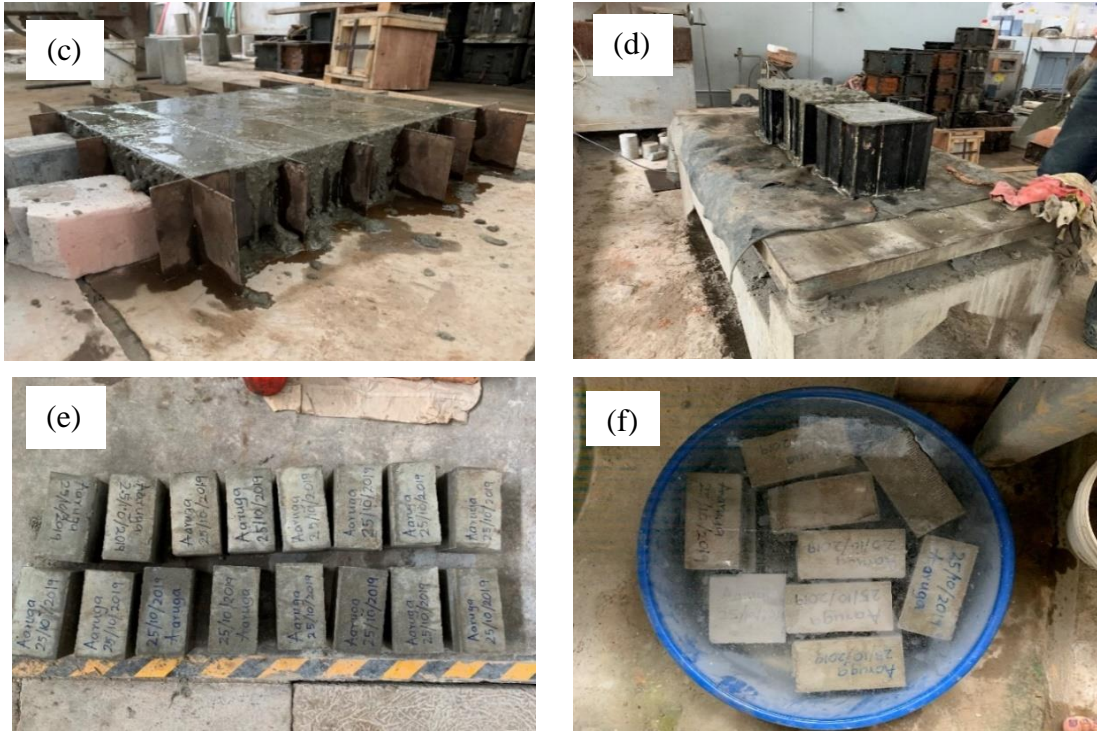
Figure 25. Preparation of concrete blocks (a) Steel formworks; (b) Applying mould oil; (c) Casting concrete blocks; (d) Mechanical compaction of concrete cubes (e) Concrete blocks after formwork removal (f) Concrete blocks during curing process
