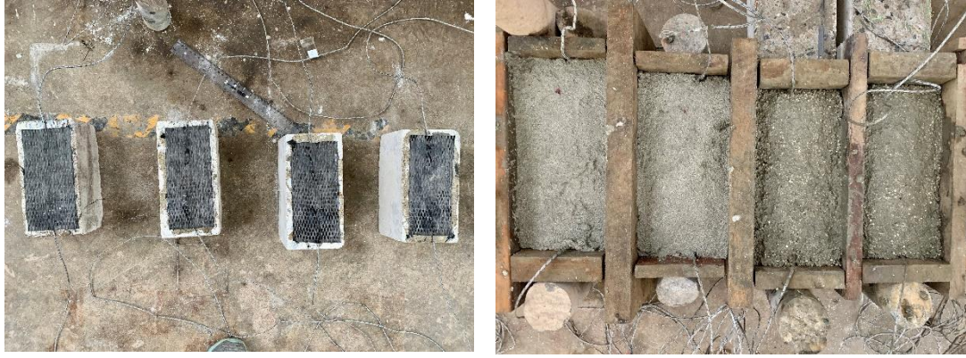
Figure 82. Application of EPS plaster as insulation for CFRP composites
