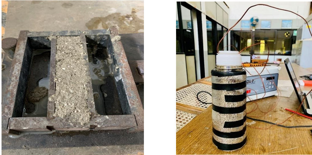
Figure 34. (a) Specimen preparation; (b) Testing of specific heat
