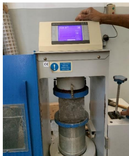
Figure 26. Testing of concrete cube strength using compressive test machine
