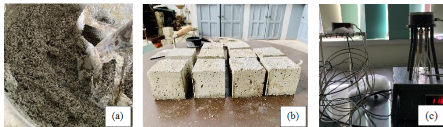
Figure 3. Specimen preparation & testing (a) Mixing mortar; (b) Compressive strength test samples; (c) Testing thermal conductivity
