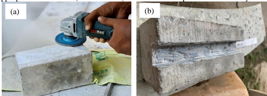
Figure 28. (a) Grinding the surface of specimen without grooves; (b) After grinding the surface of specimen with grooves
