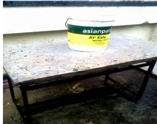
Figure 4: Glass Concrete Table Top After Applying Loads (35kg)
