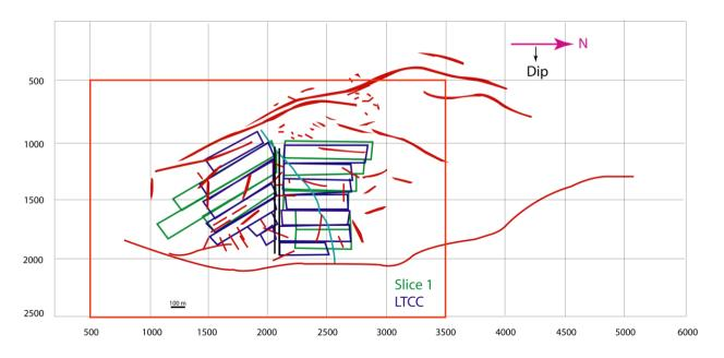
Figure. 3: The faults (red) and a dyke (cyan) of the Barapukuria coal basin and the mining panels [3].
