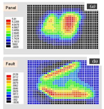
Figure. 9: The subsidence due to panel extraction with faults and the dyke effect (a) and, faults and the dyke (b).
