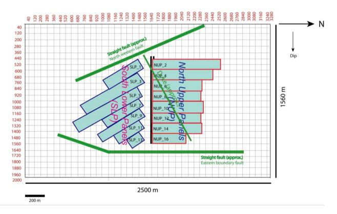
Figure. 6: The mine model with mine panels and main discontinuities.
