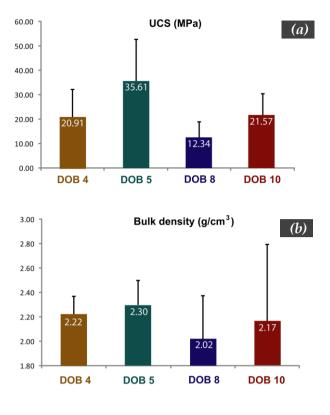
Figure. 2: The uniaxial compressive strength (a) and bulk density (b) of the rock from the coal bearing formation of the mine area.
