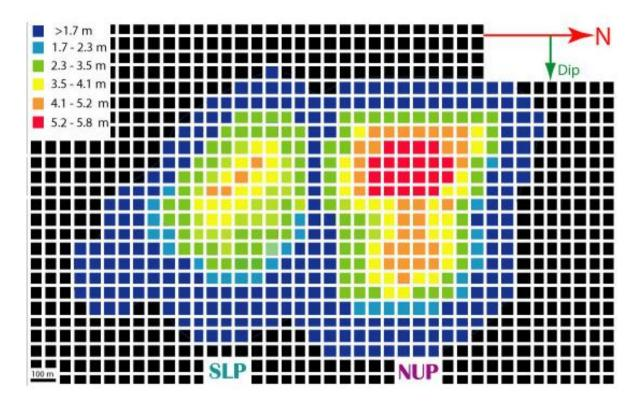
Figure. 5: The observed subsidence as grid values in the mine area.
