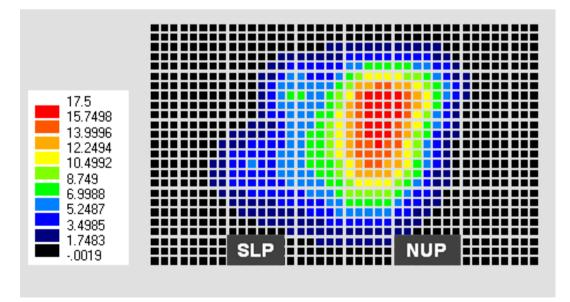
Figure. 10: Future subsidence due to total extraction of 30 m coal seam.
