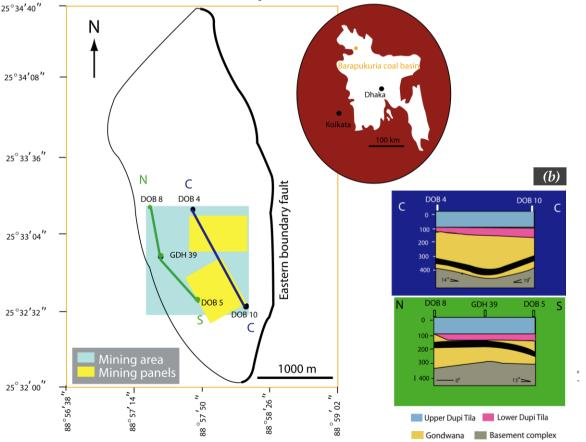
Figure. 1: Barapukuria coal basin (a) and the associated rock layers (b) with the thickest coal seam [1].
