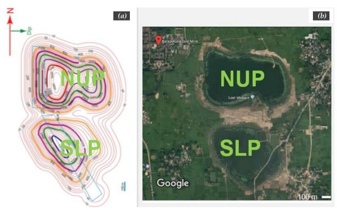
*Figure. 4: The subsidence in the mine area (a) Contour of the subsidence (b) The subsided area.*
